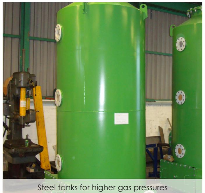
Steel tanks for higher gas pressures
